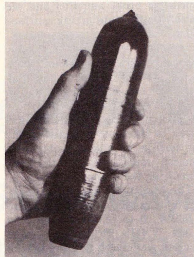
Gallium Arsenide Single Crystal Ingot
